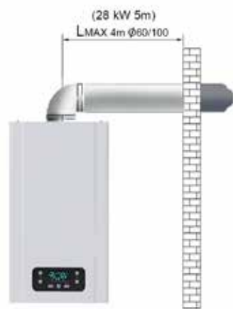
Horizontal Hermetic Flue Application L max. distance with single elbow: 4 m, Ø60/100 L max. distance with single elbow: 6 m, Ø80/125
